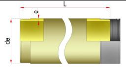
Jacking pipes with flush coupling (GRP or stainless steel), including allowable jacking forces. The standard length of the pipe is 6 m. Lengths of 1/2/3 m are available on request.
