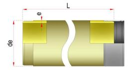
Jacking pipes with flush coupling (GRP or stainless steel), including allowable jacking forces. The standard length of the pipe is 6 m. Lengths of 1/2/3 m are available on request.
